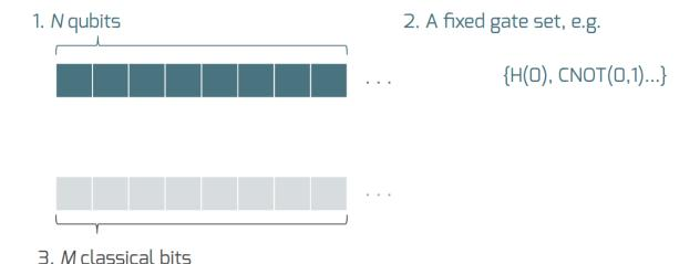
These qubits and classical bits come with a defined gate set, e.g. which gate operations can be applied to which qubits. Different kinds of quantum computing hardware place different limitations on what gates can be applied, and the fixed gate set represents these limitations.
