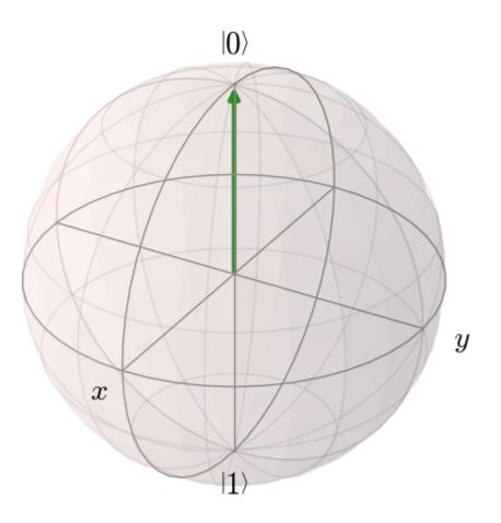
Notice that the two axes in the horizontal plane have been labeled x and y, implying that z is the vertical axis (not labeled). Physicists use the convention that a qubit's  $\{|0\rangle, |1\rangle\}$  states are the positive and negative unit vectors along the z axis, respectively. These axes will be useful later in this document.
