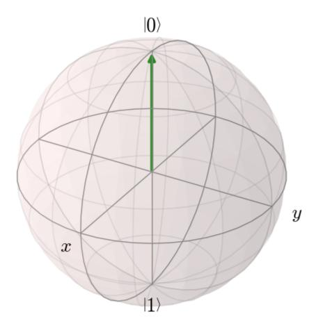
Notice that the two axes in the horizontal plane have been labeled x and y, implying that z is the vertical axis (not labeled). Physicists use the convention that a qubit's  $\{|0\rangle, |1\rangle\}$  states are the positive and negative unit vectors along the z axis, respectively. These axes will be useful later in this document.
