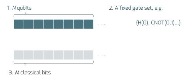
These qubits and classical bits come with a defined gate set, e.g. which gate operations can be applied to which qubits. Different kinds of quantum computing hardware place different limitations on what gates can be applied, and the fixed gate set represents these limitations.
