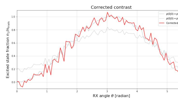
We find that the corrected signal is fairly noisy (and sometimes exceeds the allowed interval [0, 1]) due to the overall very small number of samples n = 200.
