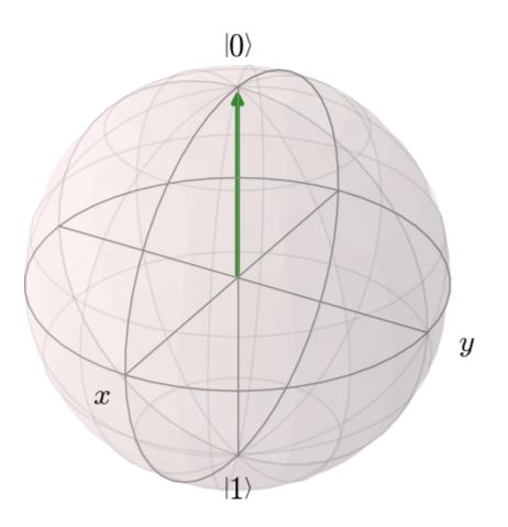
Notice that the two axes in the horizontal plane have been labeled (x) and (y), implying that (z) is the vertical axis (not labeled). Physicists use the convention that a qubit's  $((\{1,0\}, 1,1])$  states are the positive and negative unit vectors along the z axis, respectively. These axes will be useful later in this document.
