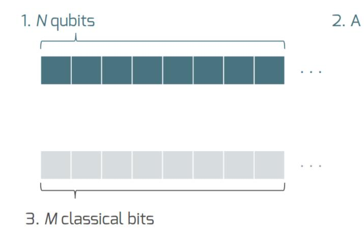
These qubits and classical bits come with a defined gate set, e.g. which gate operations can be applied to which qubits. Different kinds of quantum computing hardware place different limitations on what gates can be applied, and the fixed gate set represents these limitations.
