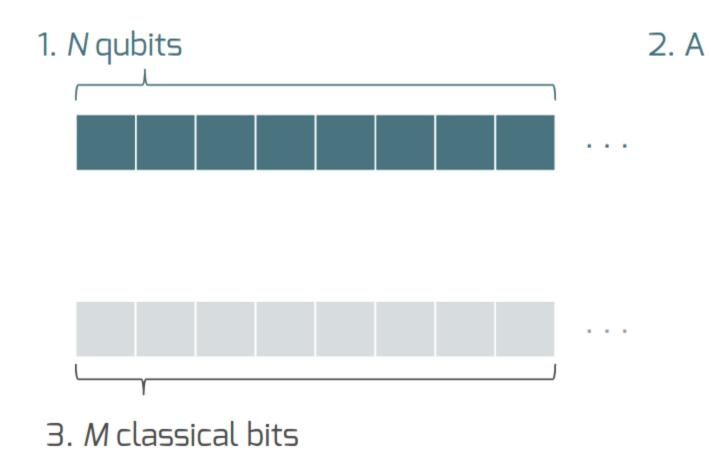
These qubits and classical bits come with a defined gate set, e.g. which gate operations can be applied to which qubits. Different kinds of quantum computing hardware place different limitations on what gates can be applied, and the fixed gate set represents these limitations.
